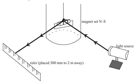
Using the magnetometer: Since many factors can affect the orientation of the magnet, including cars, tools, appliances, vibrations, etc., realize that this device is made to detect changes in the direction of the geomagnetic field and not give a quantitative measure of strength.
