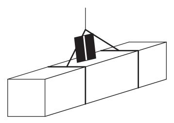
3. Glue a rectangle of cardboard to the back of the magnet to act as an air damper.
